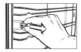
■ Remove the runners by pulling them out of the rear of the oven.
